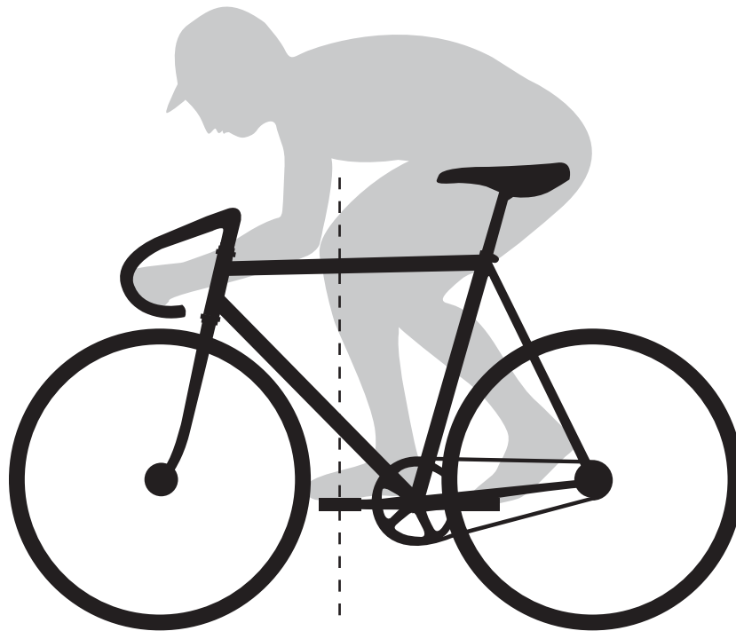
Ideally, when the cranks are level, your forward knee is directly over the pedal spindle.
