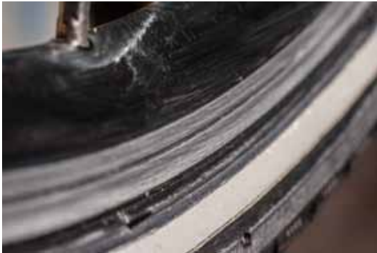
Rims require replacement when the wear line or dots disappear, or the brake surface feels concave.
