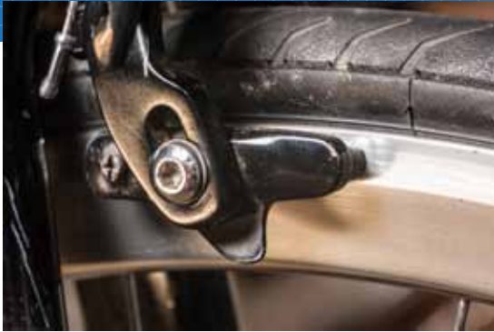
Brake pads should contact the rim in the middle of the brake surface.
